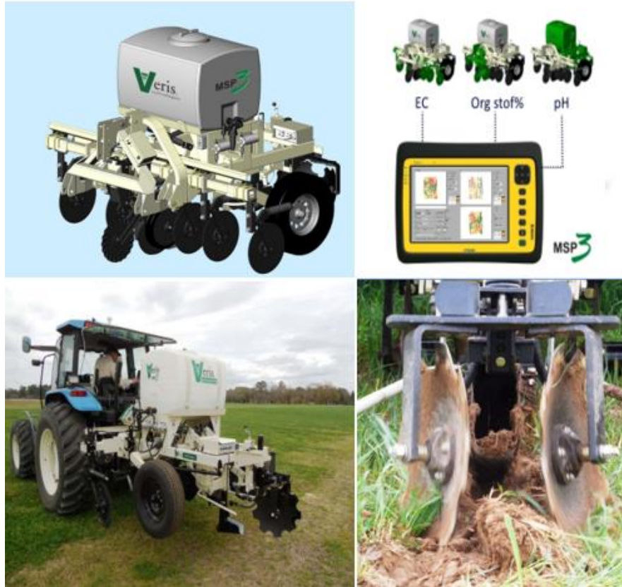
Figure 9. a) MSP3 sensor, b) pH, OM and EC coulter c) MSP3 prepared to map in the field d) MSP3 in the field (Veris Staff; Mackowiak et al., 2016).
